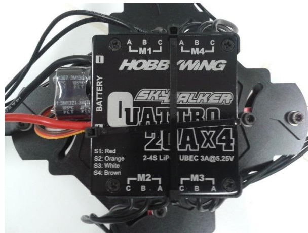
Figura 12 – ESC Hobbywing Skywalker (20A×4)
