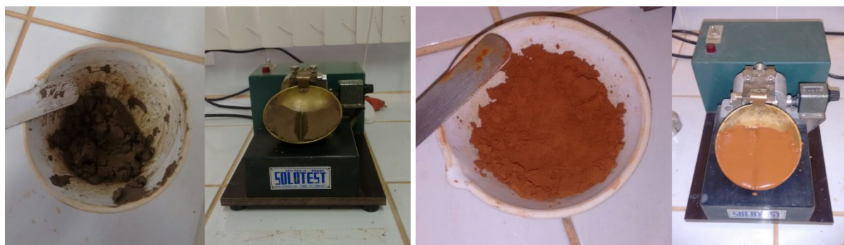
Figura 12 – Ensaios de Limites de Liquidez – Argila (a) e Chamote (b).
