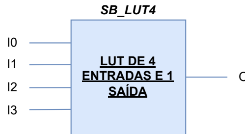
Figura 21 – LUT do Lattice ICE40UP5K.
