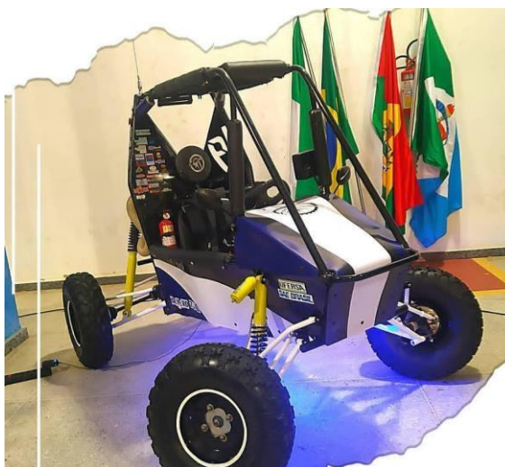
Figura 6: Chassi space frame
