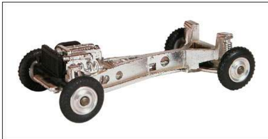
Figura 5 - Chassi Backbone (Lotus Elan)
