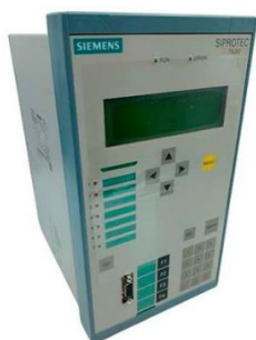
Fig. 5 - Relé digital SIEMENS SIPROTEC 7SJ622 [10]
