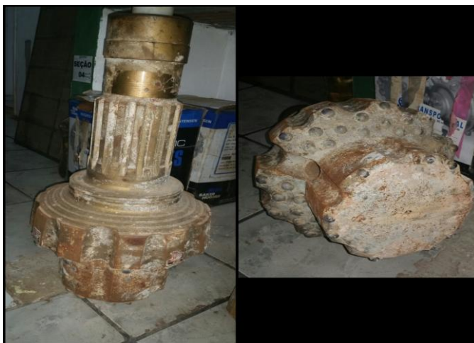
Figura 09: Bit Alargador 12 1/4" x 8 3/4"
